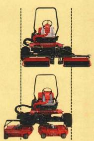
Toro® Groundsmaster® 3500-D and Reelmaster® 3100-D: Two innovative trim mowers with the Sidewinder™ cutting system. The reels on the 3100-D and the ground-following rotary decks on the 3500-D move side to side for superior trimming.
