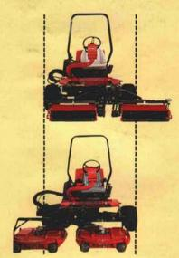
Toro® Groundsmaster® 3500-D and Reelmaster® 3100-D: Two innovative trim mowers with the Sidewinder™ cutting system. The reels on the 3100-D and the ground-following rotary decks on the 3500-D move side to side for superior trimming.
