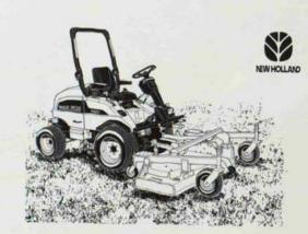
New Holland MC35 finish cut mower with 35 hp diesel engine and 84 inch deck
