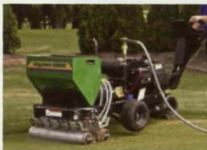
High-pressure injection (HPI) systems like this Envirojet (which has subsequently been discontinued) may be the wave of the future for effectively placing seed in a turf canopy.
