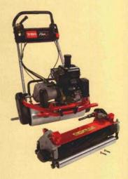
A cutting unit that comes off by removing two bolts for easy grinding and changing of reels after topdressing.
