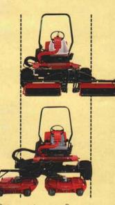
Toro<sup>®</sup> Groundsmaster<sup>®</sup> 3500-D and Reelmaster<sup>®</sup> 3100-D: Two innovative trim mowers with the Sidewinder<sup>™</sup> cutting system. The reels on the 3100-D and the ground-following rotary decks on the 3500-D move side to side for superior trimming.
