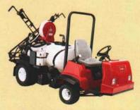
Toro<sup>®</sup> Multi Pro<sup>®</sup> 1200 and 1250 sprayers: Featuring the innovative Spray Pro<sup>™</sup> control system that directly links flow rate to ground speed ensuring precise application rate.
