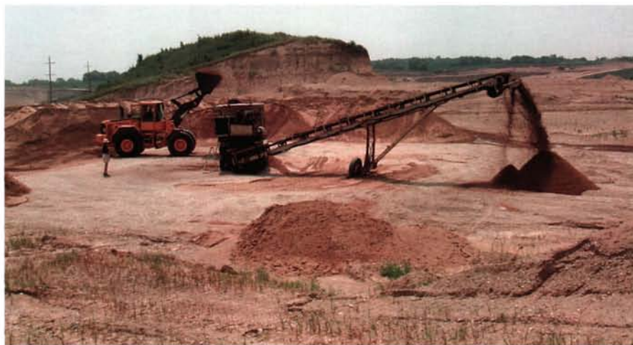
Inspecting the blending site for a hard surface during prequalifying visits to local sand suppliers is necessary to prevent contamination of the root-zone stockpiles once produced.
