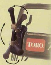
A single control lever to engage both the traction and reel.
