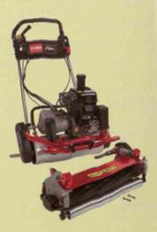
A cutting unit that comes off by removing two bolts for easy grinding and changing of reels after topdressing.
