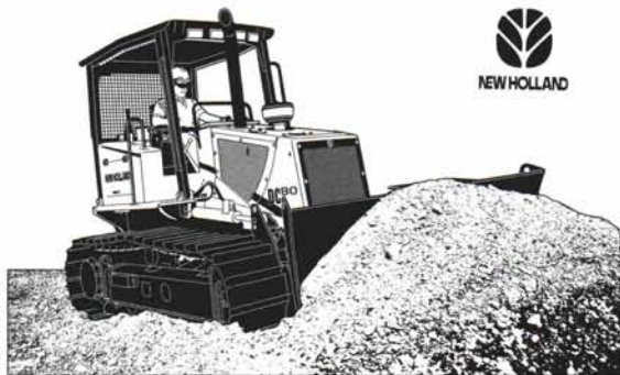
80 hp dozer with hydrostatic transmission and 9'4" blade
