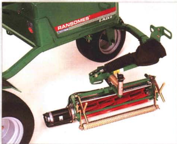
Rear cutting unit swings out for easy access.
