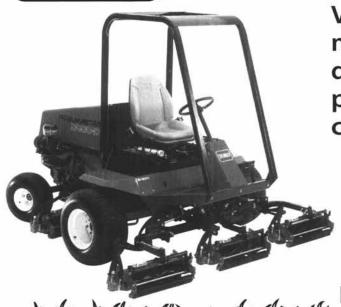
Variable speed fairway mower provides a superb quality of cut with two powerful diesel engine choices - 28hp or 35hp.
