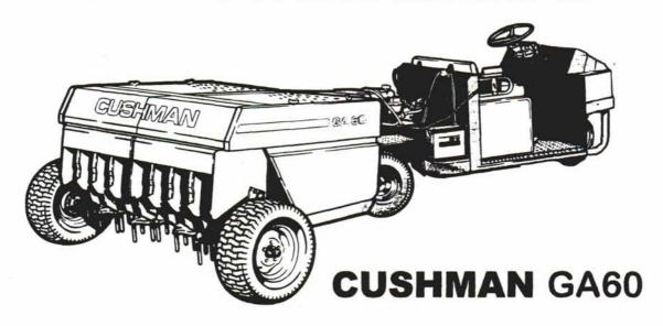
Full 60-inch aerator with eight timed and balanced aerating heads for greens-caliber aeration, governed rotation speed for maximum productivity with minimum plant/soil disturbance.
