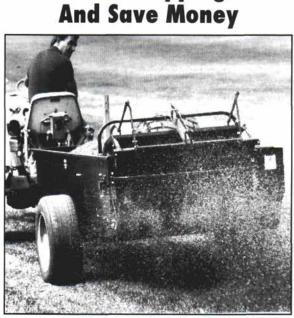
In one easy step, eliminate costly dumping fees and improve the rough by spreading grass clippings still enriched with precious fertilizer. Millcreek's Top Dressers are equipped with an adjustable undershot poly brush designed to evenly distribute top dressing from three to ten feet wide.
