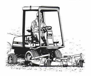
Ford commercial front mowers make fast work out of big jobs. Hydrostatic rear-wheel steering, independent right- and left-hand brakes and a clutchless shift from forward to reverse makes your job easier. Stop in and put one to the test.
