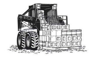
The New Holland Super Boom™ skid-steer loader will help you be more productive no matter what the application. The long wheelbase makes it more stable so you get better lift capacity than ordinary loaders. And it can go uphill with an empty bucket and come down with a full one.
