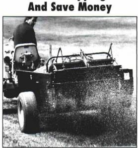
In one easy step, eliminate costly dumping fees and improve the rough by spreading grass clippings still enriched with precious fertilizer. Millcreek's Top Dressers are equipped with an adjustable undershot poly brush designed to evenly distribute top dressing from three to ten feet wide.
