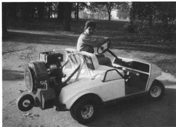
Joel Purpur sent this photo in on a quick way to mount a 16 h.p. Billygoat Blower to a golf cart. Take off the wheels and handle — clamp it on and away you go. Greens, tees, and fairways are able to be blown without getting tired.
