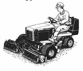
2653 cutting units feature a quick height of cut adjustment system that enables changes to be made at 1/8 inch intervals.
