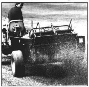
In one easy step, eliminate costly dumping fees and improve the rough by spreading grass clippings still enriched with precious fertilizer. Millcreek's Top Dressers are equipped with an adjustable undershot poly brush designed to evenly distribute top dressing from three to ten feet wide.
