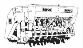
SIMULTANEOUSLY REJUVENATES, AERATES, FERTILIZES AND SEEDS IN ONE PASS. ALSO THE IDEAL MACHINE FOR PLANTING ORIGINAL SEEDBEDS.
