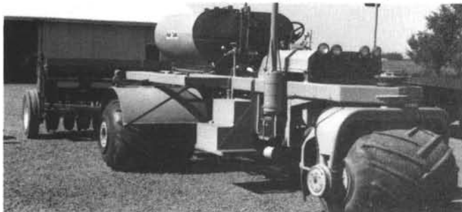
6. Another "Rubber Duck" with the seed disc behind. The tank would hold the charcoal slurry to be sprayed over the seeded rows.
