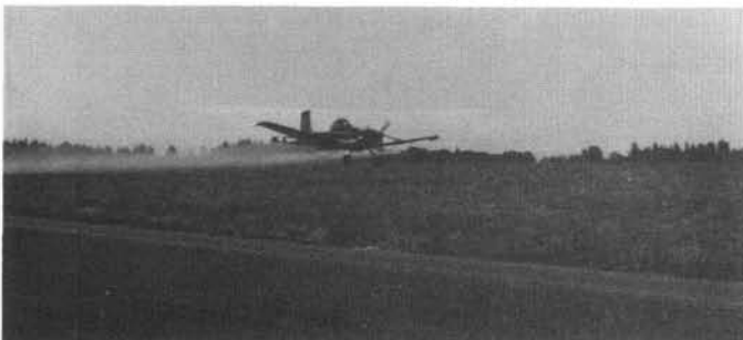
8. A crop spraying plane that sprays 5 gallons per acre and can do 40 acres per load. The plane has a 275-gallon capacity.
