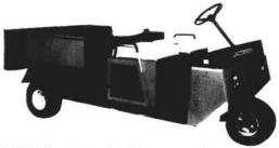
**T2000** - The T2000 is a durable, tough, low-maintenance vehicle that is really looking for work. And work it does, with the capability of hauling, seeding, top dressing, aerating, spraying, and can be utilized for the 100 and 1 other jobs where a good turf truck is needed. Total vehicle capacity is 2,000 pounds.
