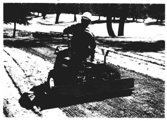
Spring-loaded box scraper and scarifier with closed ends prevents windrows. Automatically self-relieving across entire width of scraper to leave a smooth, even surface.
