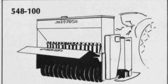
3 pt. mount PTO Drive Overseeder Front half can be used as a detachable forward reverse gear box.
