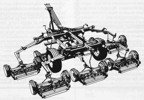
The Reelmaster™ Transport Frame from Toro: Features hydraulic arms that lift 7 reel mowers in various combinations for amazing maneuverability around benches, trees, other obstacles. Plus,
