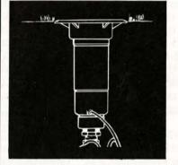
consistent rotation. Toro's exclusive valve-in-head feature prevents low head drainage and valve is serviceable without digging.
