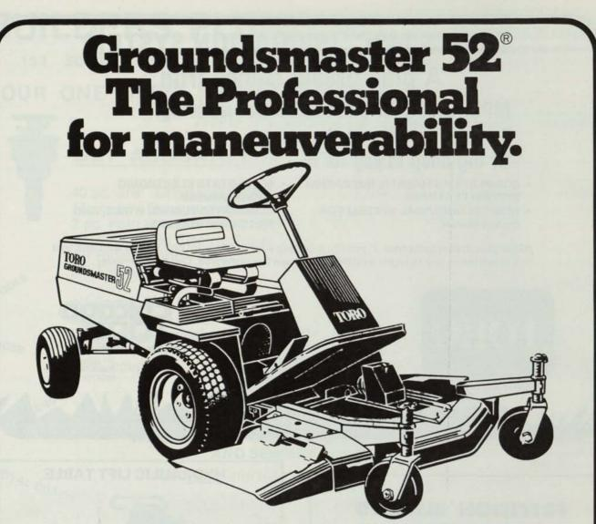
The Groundsmaster 52<sup>®</sup> offers wide cutting ability. It trims tight around trees and other obstacles with the offset, forward mounted 52'' deck. One
