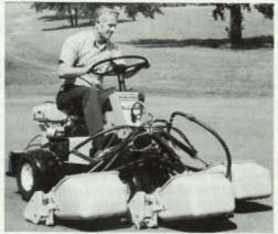
When you have finished mowing your greens . . . In less than a minute, you can change the Greens Cutting heads for the Verti-Cut Units to remove thatch and grain . . . Or attach the Vibra-Spiker heads and achieve deep spiking penetration without excessive weight, and eliminate the back-breaking ordeal of "summer-aerification" . . Or attach the heavy-duty Utility Units which are ideal for approach and tee mowing, or they can be adjusted down for greensmowing after top dressing.
