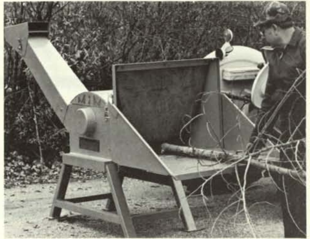
Mitts & Merrill Brush Chipper designed for Golf Course use. Uses P.T.O. Power and 3 pt. Hitch for economical price and operation.
