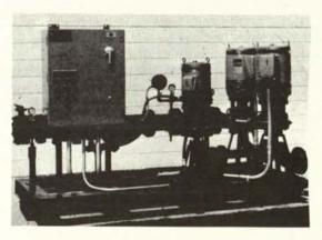
The two main pumps are Cornell 40 h.p. or 50 h.p. units. Total unit capacities range from 750 to 1200 GPM at pressures of 100 p.s.i. to 118 p.s.i. Other ranges available.
