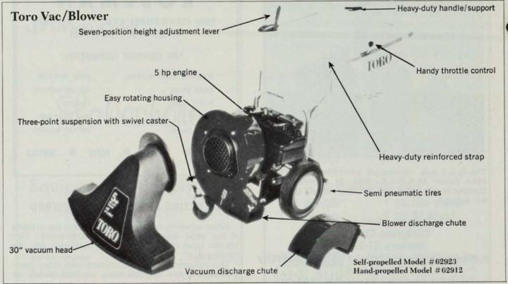
Toro Vacuum-Blower: Toro has equipment that helps you gather debris quickly and easily. You can pick a Toro Vacuum-Blower that is hand-propelled or one that is selfpropelled. Both convert from vacuum to leaf blower in less than five minutes without costly optional equipment or tools. Each holds up to seven bushels of leaves; has fittings for an optional extension hose that gets even the most stubborn bits of debris out of bushes, hedges, window casements and other tough places.
