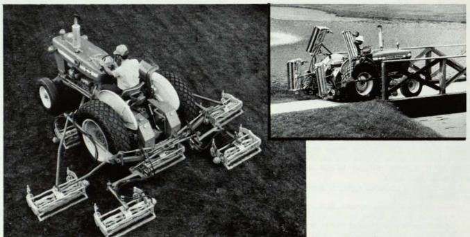
Beginning a new era in turf mowing, the Roseman 7 unit Hydra-Gang Mower utilizes the tractor power takeoff system to power the cutting reels and the tractor hydraulic system to provide hydraulic lift for each mower unit. Hills and banks can be mowed easily regardless of soft or wet turf conditions. Individual mower units follow ground contour with unlimited flexibility without scalping. The Hydra-Gang mounts on Ford 2000 and 3000 All Purpose model tractors.
