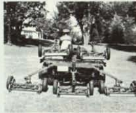
FIVE-UNITS: Over-all width approximately 12'2". Cutting width about 11'.
