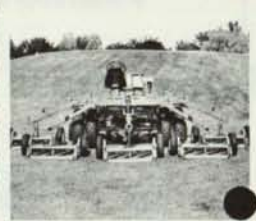
SEVEN-UNITS: Cutting width about 15', over-all width is approximately 16'2".
