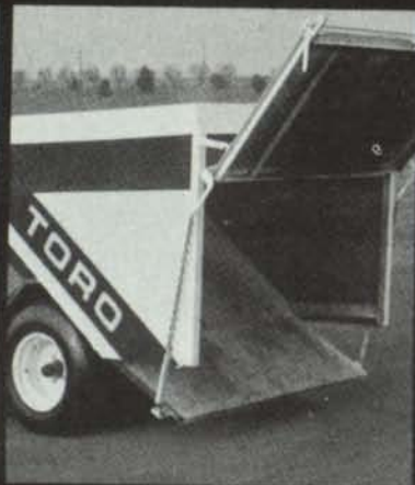
FULL-WIDTH GATE and sloping floor give fast unloading of 115 cu. ft. hopper. Airstream carries litter to rear of hopper so there's no wasted space.
