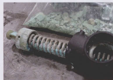
Mixing and keeping your solution in suspension is important. There are many items like this flow valve that solids can accumulate on and clog the system.
