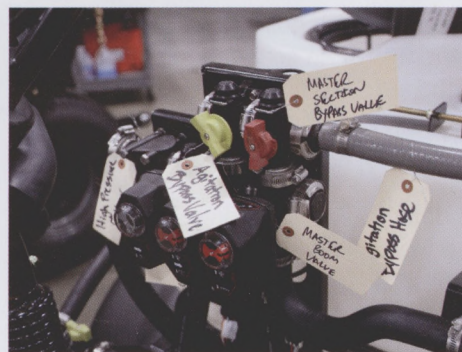
Reinders took the time to label all the parts on a sprayer they had in the shop.
