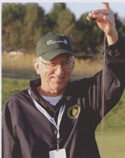
In the early days of firmness testing, a steel ball was dropped from about head-high onto a putting surface and the depth of the indentation was measured.
