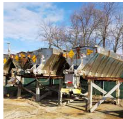
The spreaders get a rest during the warm months when the trucks are converted back to regular dumps.
