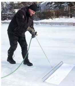
A resurfacing flooder is nothing more than a small boom sprayer with a material attached to it that helps to level and smooth the ice.
