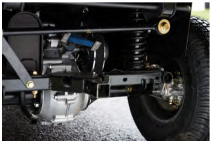
Coil-over shocks suspension for smooth operation
