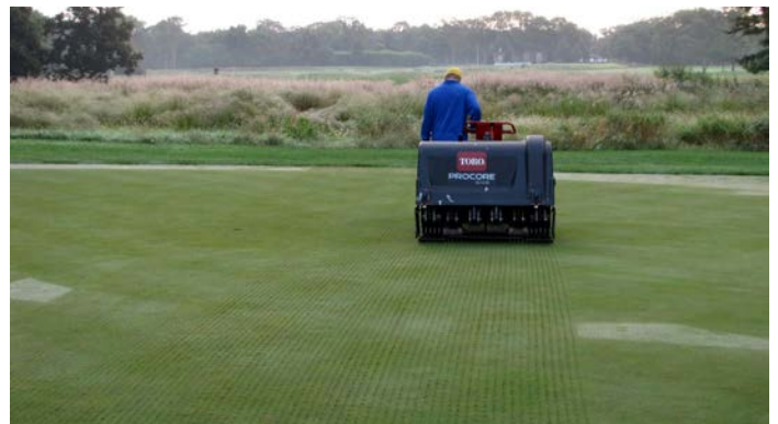
When the opportunity arose, many superintendents began to groom. Small solid tines were used on the turf above - less detrimental to weakened turf than large hollow ones.
