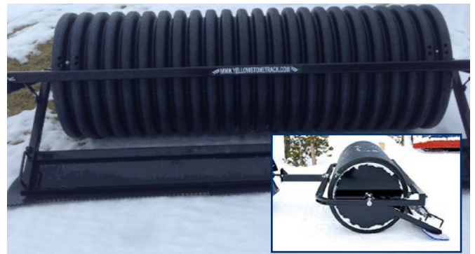
I follow the rough trail I've set with the snowmobile pulling the roller/compactor setting the trail in place.
