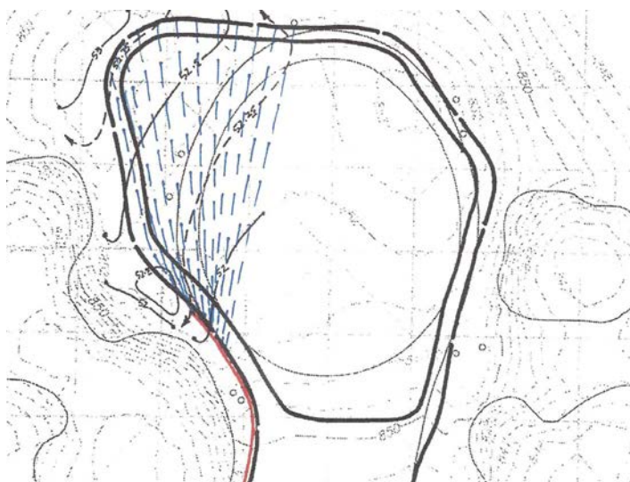
This is a drawing from North Shore's 13th green that shows the PC element (blue lines) and where it will connect to the existing drainline (red line).
