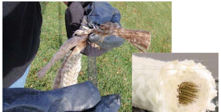
The PC element is a stainless steel mesh tube shrouded by woven fiberglass.
