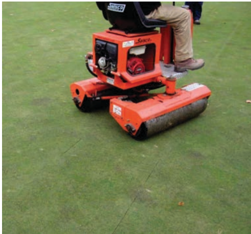
A little rolling over the slits from the plow and the area is ready for play.
