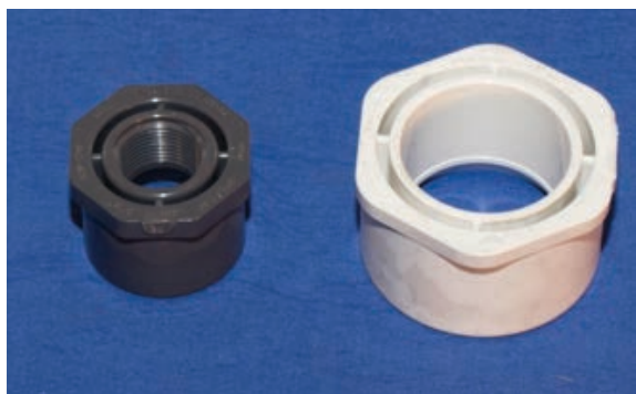
PVC pipe fittings come in many sizes, threads and schedules. Schedules are used to describe the thickness of the walls. Schedule 80 is thicker than 40 and can withstand higher pressures.
