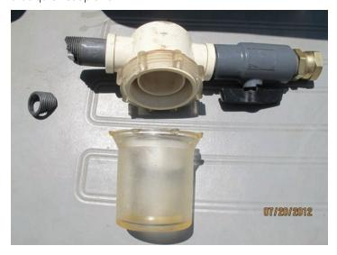
When pressure reached this applicator, the jar broke just under the threads, hurtling it 63 yards from its operator, with an accompanying pop heard over 400 yards away. The nozzle
