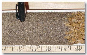
The gravel however is a different story. This course is in an area where bridging gravel is very scarce and expensive to haul. So, instead of adding an 'intermediate layer' with a choker sand/gravel that would have separated the mix from the drainage gravel, the builder simply placed the mix on the locally
