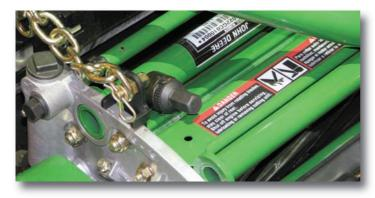
The QA7 has 1-click reel to bedknife adjustment as well as the new HOC adjustment. The 22 inch reel comes with 8 or 10 blades and is for the 7700 and 8700 fairway units. The 26 and 30 inch come with 5 or 8 blades and are available on the 7200 and 2653B trim/surrounds units.
