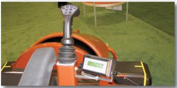
The guys from Finland brought their mower, the "ONE". Lithium-ion battery pack that lasts 7-8 hours. Plug in the wall recharging. Auto HOC and FOC. Auto clipping dispersal. No steering wheel, no pedals. AC servo motor drives. One hand joystick operation. Programmable control systems via satellite antenna with Finland. A 4 wheel fairway unit with 5 or 7 cutting units and a walker are scheduled to be released later this year.
