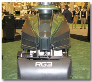
The 36V lead-acid battery supply is segregated; 24V for the mower operation and 12V for the software. The software is loaded onto your computer at work. You set the mowing schedule (days of week), parameters (single or double cut), direction, cleanup, and the distance it goes **after** it leaves the green before it makes its turn. Cleanup is accurate to within ½ inch.
