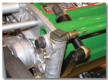
Also new are the cast aluminum side frames. The QA5 comes in 18 inch width for the 8000E fairway mower and 22 inch width for the 220E walker, 2500B, and 2500E triplex greensmowers. The 7500, 7500E, 8500 and 8500E fairway units also contain a 22 inch width. Seven and 11 blades are available.
