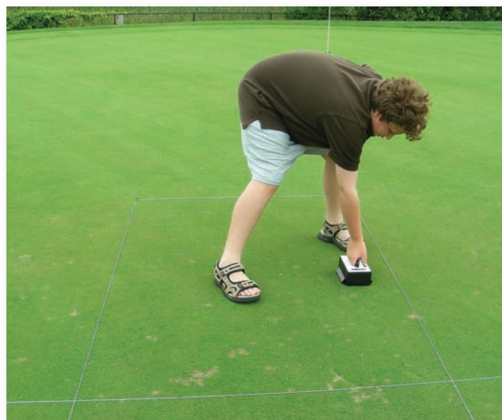
Figure 3. NDVI was used to capture light reflectance of red and near-infrared wavelengths to quantify chlorophyll content of a bentgrass green.
