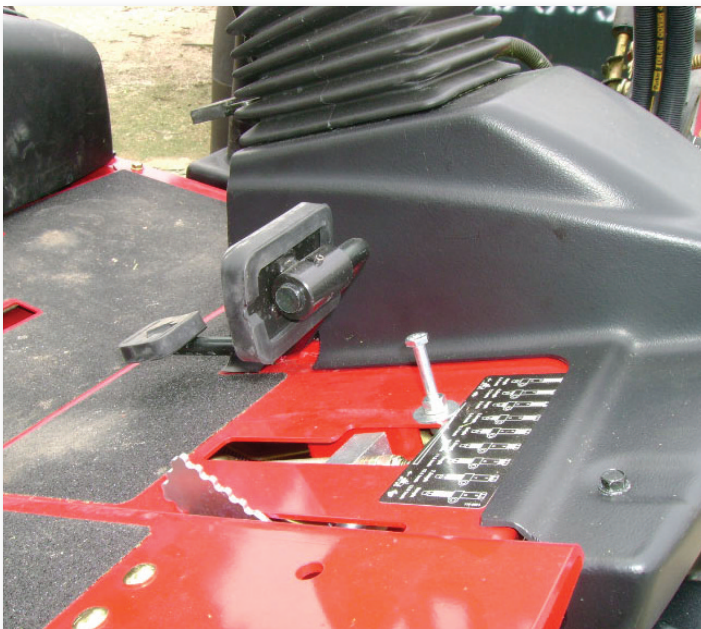
Toro RM5210 uses a pedal stop that is fully adjustable. The installed bolt controls the amount of pedal travel to keep the machine at a safe and controllable speed.
