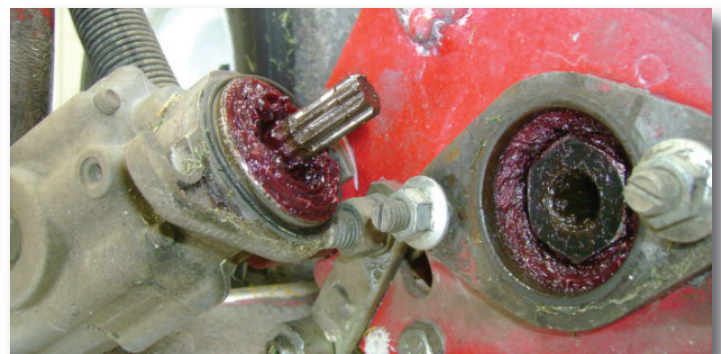
Below: For a few pennies, a slim o-ring will create a water tight seal between the reel motor and reel bearing housing.
