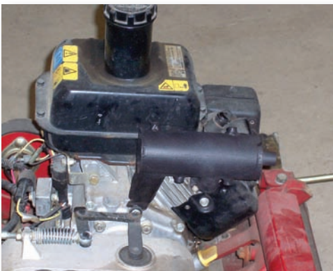
The Image below is the Smog Avenger™ installed on a Toro Flex 21 mower at Mistwood Golf Course. Heat shield is removed for image.
