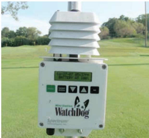
Figure 2. Close-up of the mini weather station with a light sensor used in this study.
